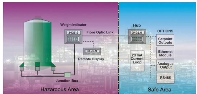
This third example shows a fibre optic link between the hazardous area and the safe area. Full functionality of the ATEX certified Weight Indicator is available through the Hub Terminal in the safe area and an extensive range of communication options complete this flexible and versatile installation. Power to the instrumentation in the hazardous area may come from certified batteries or mains supplies.
