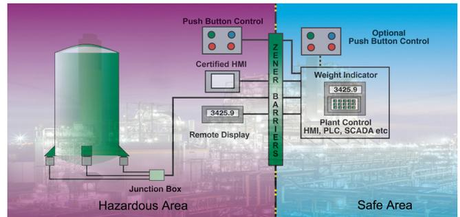
In this conventional hazardous area weighing application, the system integrity is maintained via Zener Barriers. Optional ATEX certified equipment such as remote weight displays or HMIs can be located in the hazardous area, powered from the safe area via the Zener Barriers. Control functions are typically carried out from the designated safe area.
